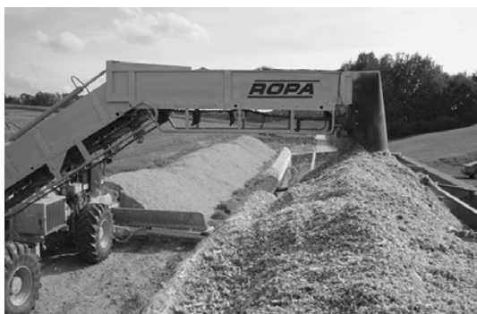
Sl. 3 ROPA NawaRo-Maus stroj za pretovar krme s polja u velike prikolice Fig. 3 ROPA NawaRo-Maus machine for loading silage from field to trailers
