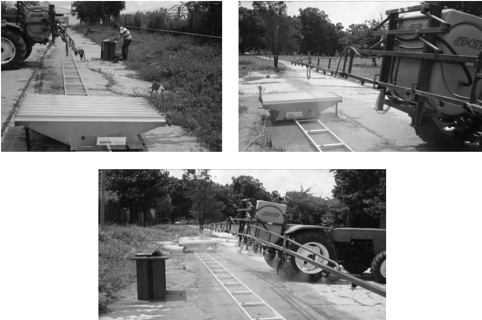
Fig. 3 Transversal distribution uniformity determination for new/used nozzles - aspects during measurements
