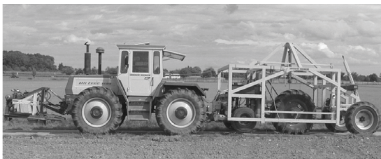
Figure 2 Single wheel tester based on a measuring trailer [6]
