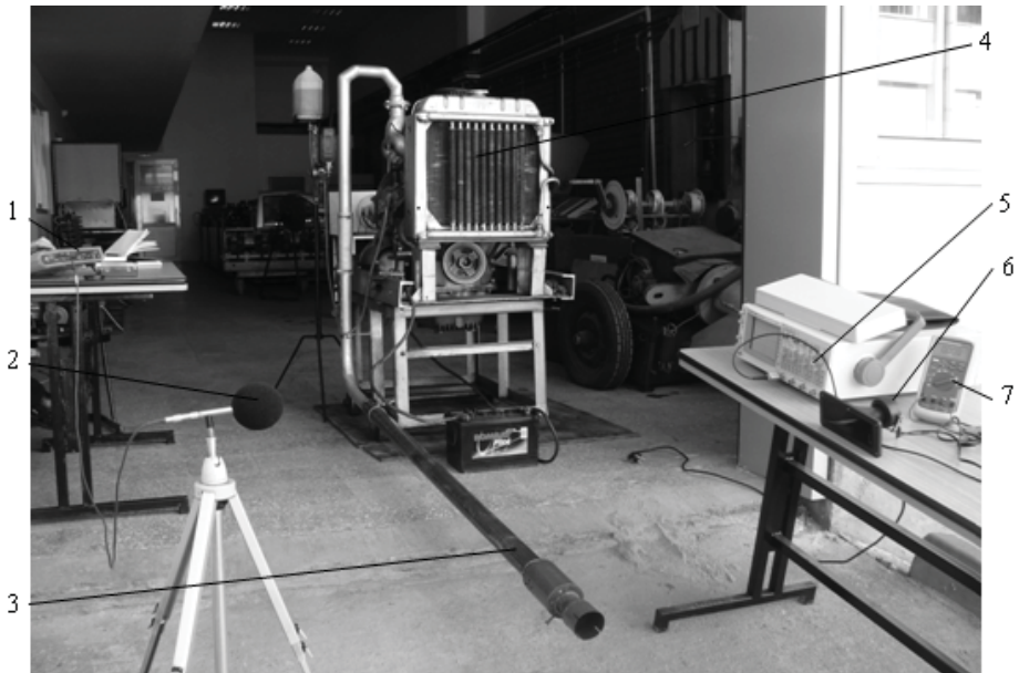
Figure 3 The experimental stand for noise energy conversion evaluation; 1 – N 121 noise analyzer; 2- microphone; 3 – exhaust pipe; 4 – D 30 Diesel engine; 5 – oscilloscope; 6 – tweeter SAL KHS110 (acoustic transducer); 7 – energy supply measurement instrument
