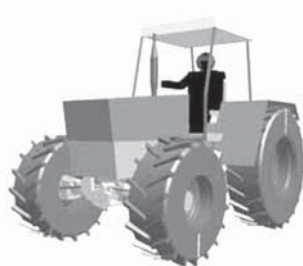
Figure 1 Graphical representation of the tractor modeled as multi-body dynamic system [1]
