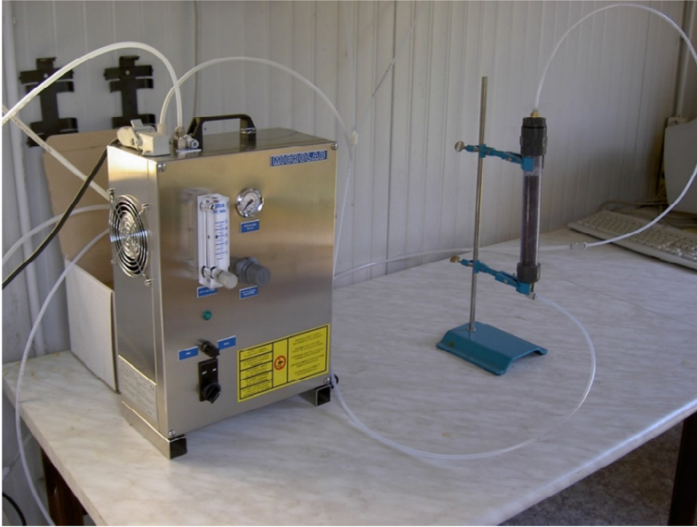
Fig.1. The ozonator linked to the column, used for the simple test [6]
