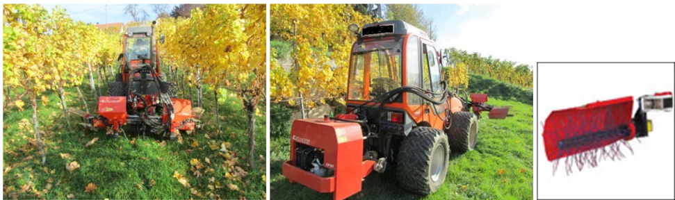
Figure 1: Lotti IT 26A platform during operation (left) equipped with CP21 pump unit (middle) and TRF50 cutting head (right)
