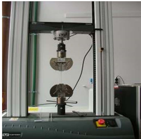
Figure 1. Tensile test of sample with TPS matrix on Instron 3360 Series
