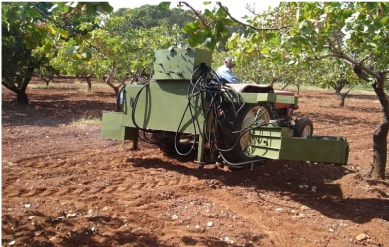
Fig. 2. Orchard tests with body shaker
