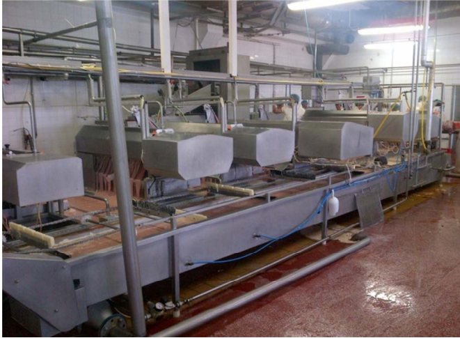
Figure 1 - Hog Casing Cleaning Line (with 6 machines).
