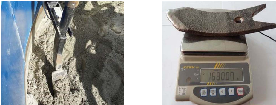
Fig. 11. Aspects from determining the wear of chisel type active bodies
