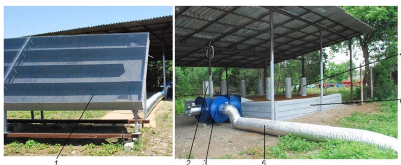
Fig. 2 Experimental model of installation for fodder aeration
