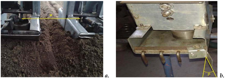
Fig. 6 - The parameters of the pads a. w -distance between the pads' wings axis; b. \beta -wings angle with the motion direction
