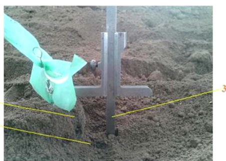
Fig. 9 Measuring planting depth
