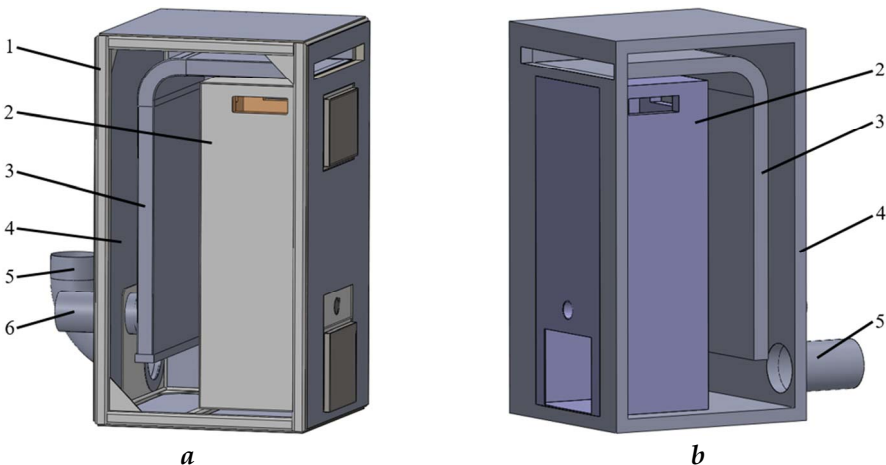
Figure 2 Greenhouse heating equipment (lateral wall removed): (a) isometric view; (b) simplified view, for CFD simulation; 1 – steel frame; 2 – TLUD module; 3 – heat exchanger; 4 – insulated exterior wall; 5 – flue gas evacuation; 6 – hot air pipe.
