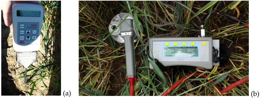
Figure 1. Soil temperature, electrical conductivity (a) and CO 2 emission rate (b) portable measuring devices (Buragiene et al., 2015).
