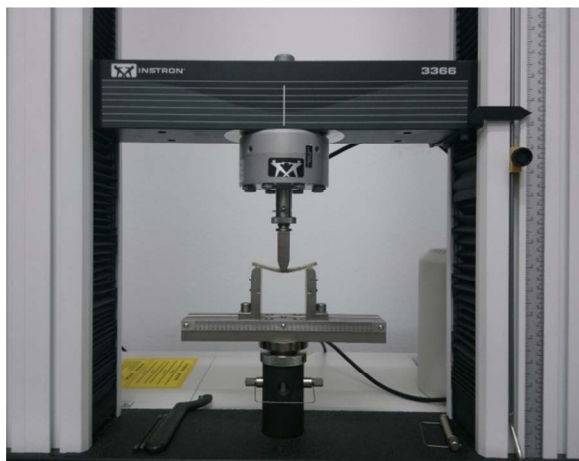
Figure 2. Bending test of sample with PBAT matrix on Instron 3360 Series
