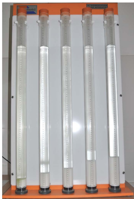
Fig. 3 Laboratory stand W2 Sedimentation Studies Apparatus – Armfield Limited
