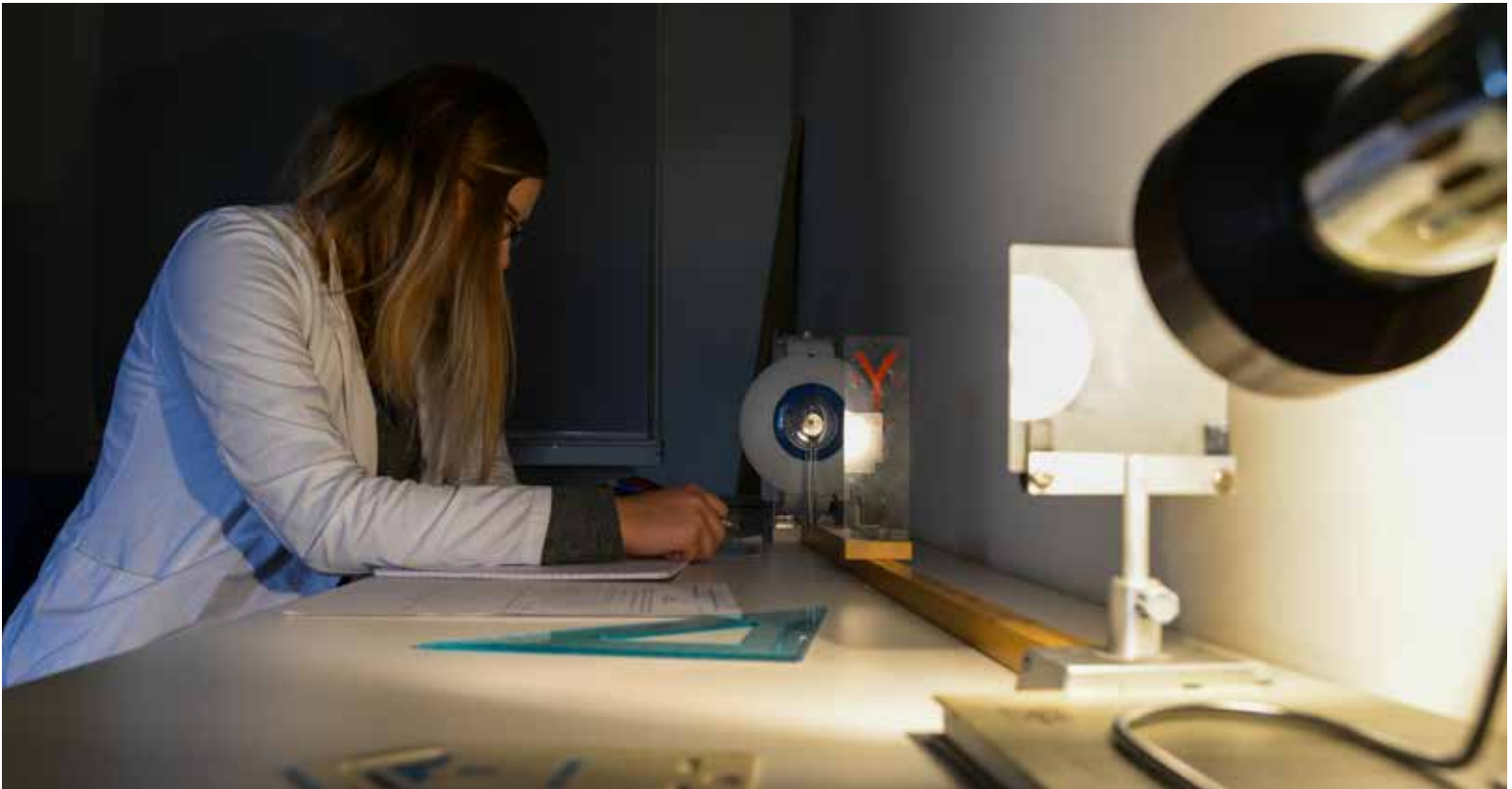
One part of the Physics Practicum takes place in two darkrooms. In this photograph: a human eye replica with the source of light and an object, on which students can study accommodation and refractive errors, e.g. nearsightedness (myopia) and farsightedness (hyperopia).
