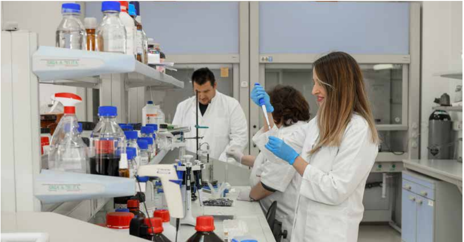
Members of the Department performing analysis of ether extract content in corn silage samples in the Laboratory for Safety and Quality of Animal Feed. Ether extract analysis is a part of the proximate chemical analysis (Weende method) used for the feed quality assessment.
