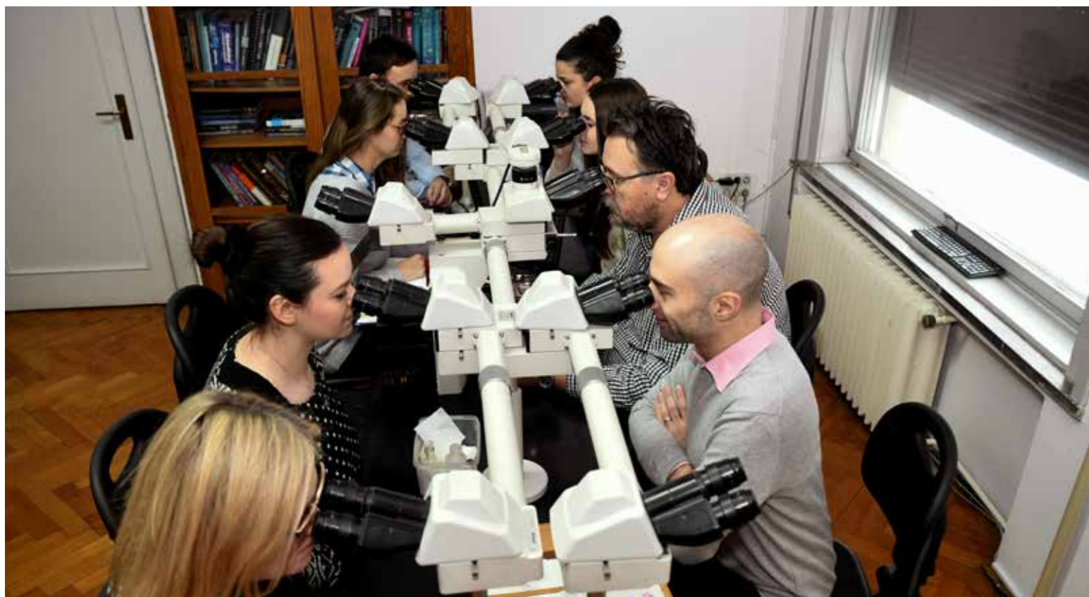
Allowing multiple users to observe the same specimen using separate eyepieces, the discussion microscope system is ideal for both teaching and consulting, as well as for reviewing difficult cases with other pathologists and colleagues, and discuss the diagnoses.
