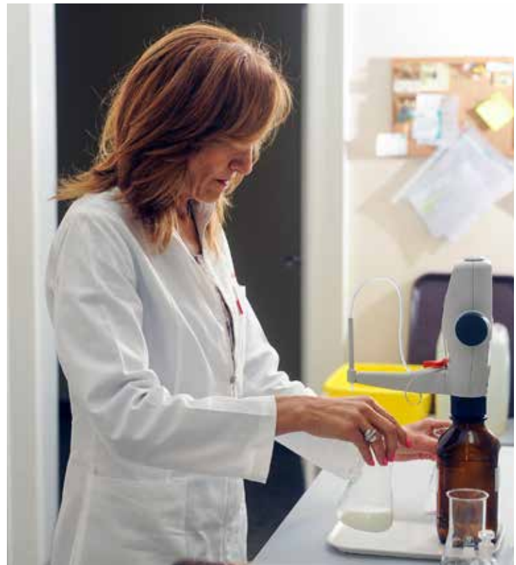
Quality evaluation of food of animal origin is carried out within the professional and scientific-teaching part of work. In this photograph: determination of the freshness of milk by titration.
