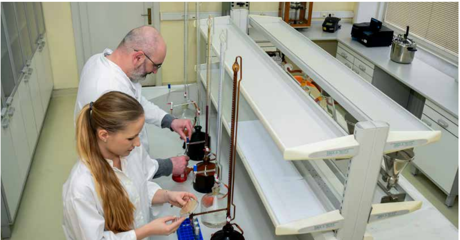
Measurement of the consumption of potassium permanganate (KMnO 4 ) in a laboratory, a parameter indicating the amount of organic matter in the water. Water containing the organic matter (contamination) of human, animal or industrial origin will use a certain amount of KMnO 4 for its oxidation.
