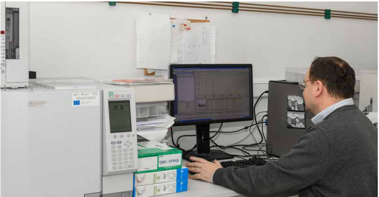
Investigation of lipid metabolism is regular scientific activity of Department of Animal Nutrition and Dietetics. Fatty acids and their metabolites are investigated using gas chromatography with mass detection.
