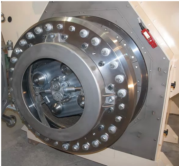
Figure 1 Die Exchange System – QDES.60 (Cenei Industrial Park)
