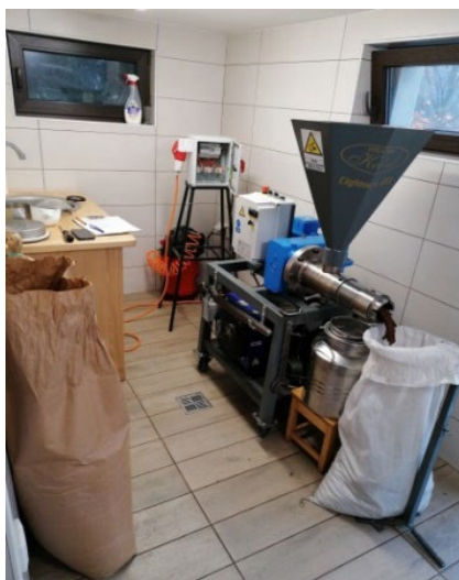
Figure 1 Mechanical extraction of vegetable oils with screw type press in a small oil mill on family farm, measuring equipment for determining electricity consumption of rape seed pressing is connected with the screw type press.
