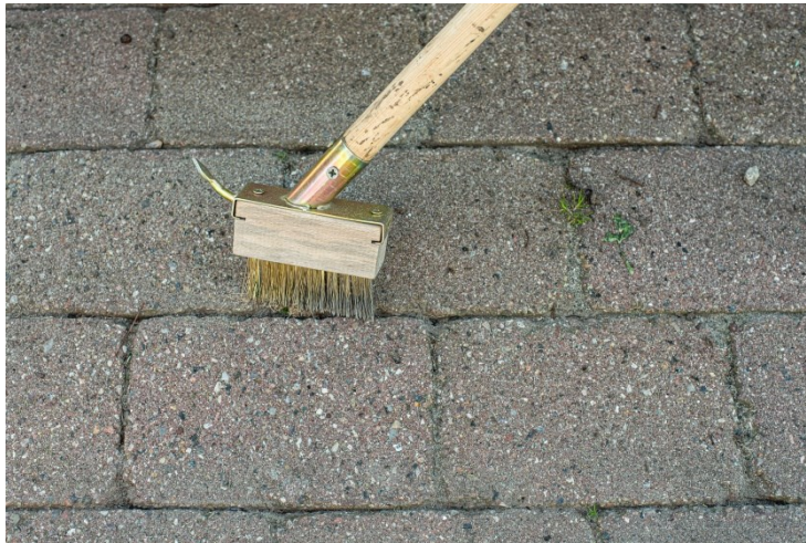
Figure 5.19 Brush weeder ( https://www.shutterstock.com )
