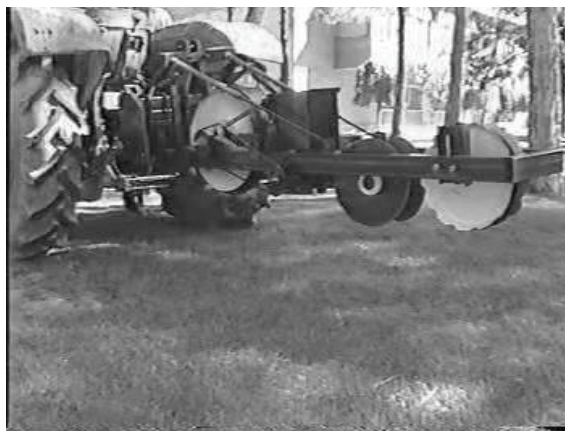
Fig. 1 Constructed planter mounted on tractor
