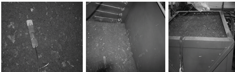
Figure 1 The force sensor Flexi Force applied on soil before being covered by soil and to the depth of 75 cm and after it was covered to the depth of 5 cm
