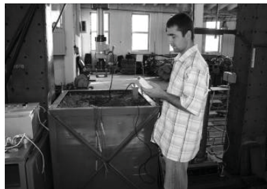
Figure 3 The tests command centre and the soil humidity measuring with humidometer type HH2
