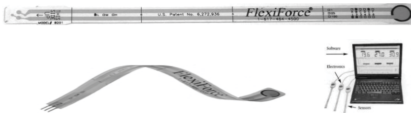
Figure 4 Force sensor Flexi Force, Laptop and acquisition system
