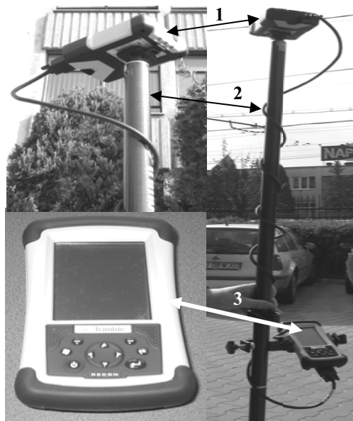
Fig. 1 The Trimble GPS device: 1 – receiver and antenna; 2 – handling stick; 3 – recon with display for setting the operation system
