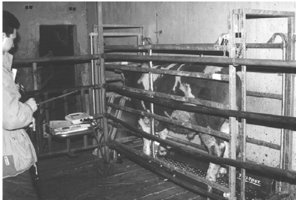
Fig. 2 The animal stands on a platform. The entrance and exit gates are not connected to the platform and therefore are not weighed
