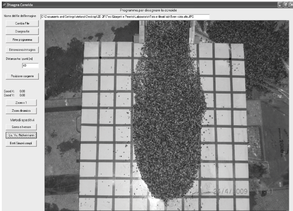
Figure 2: Experimental set-up for 2D debris flow propagation studies
