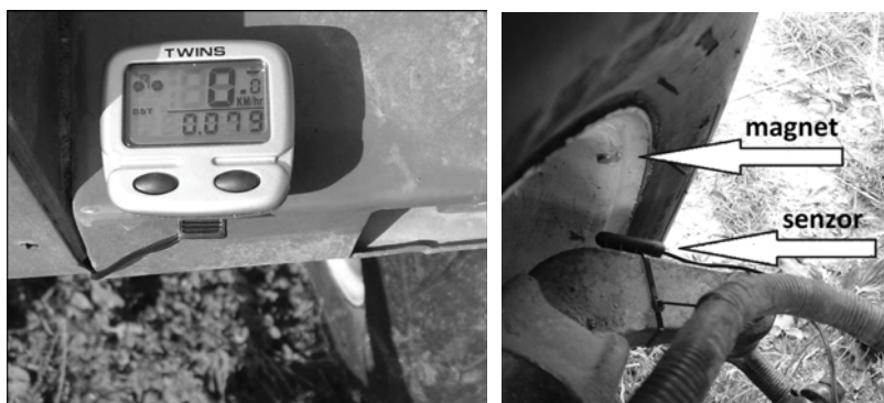
Figure 2 Cycling counter fixed on the dashboard (left), installation of sensor and magnet on the wheel (right)
