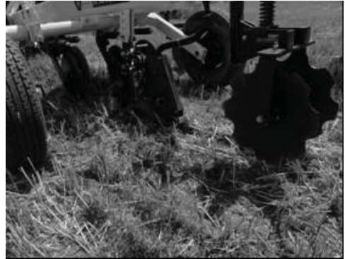
Fig. 4 Detail shank with optical sensor
