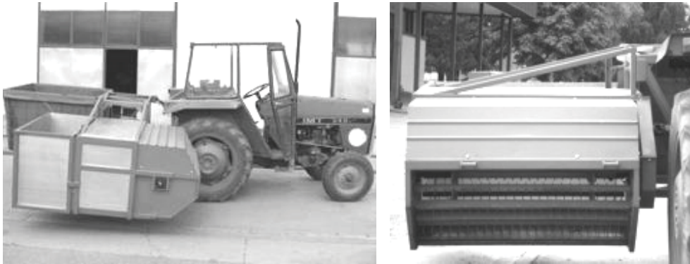
Fig. 5 Tractor mounted harvester, virtual rotated comb type, used for mechanical harvest of marigold flowers
