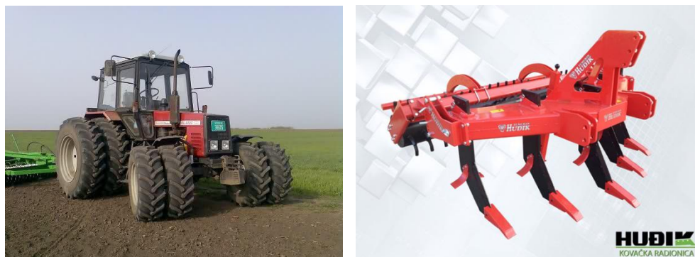
Figure 15 Typical measure of soil pressure abatement, twin-tyres on Belarus tractor (left); Low depth subsoiler combined with rotary harrow for plough pan elimination (right)
