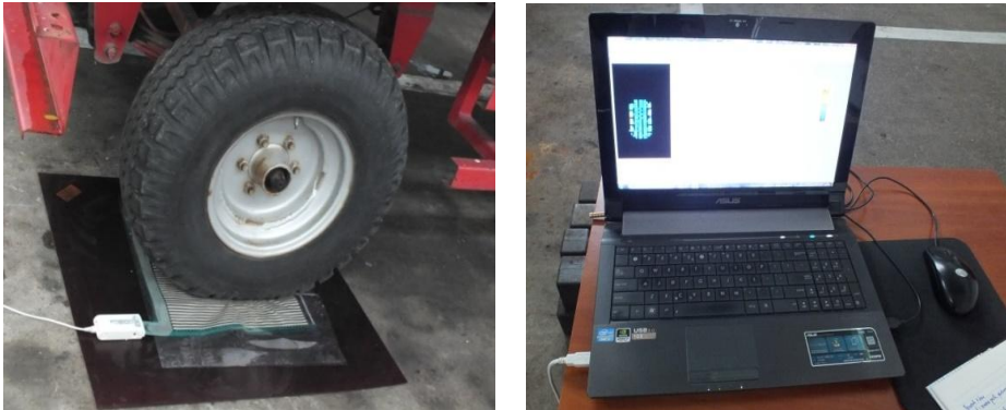
Fig. 3 Connection of sensor to the data acquisition system and laptop
