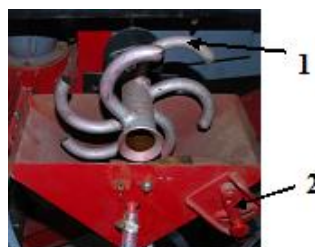
Fig 3 Liquid dispenser 1- dosing system with tubes 2- adjusting system
