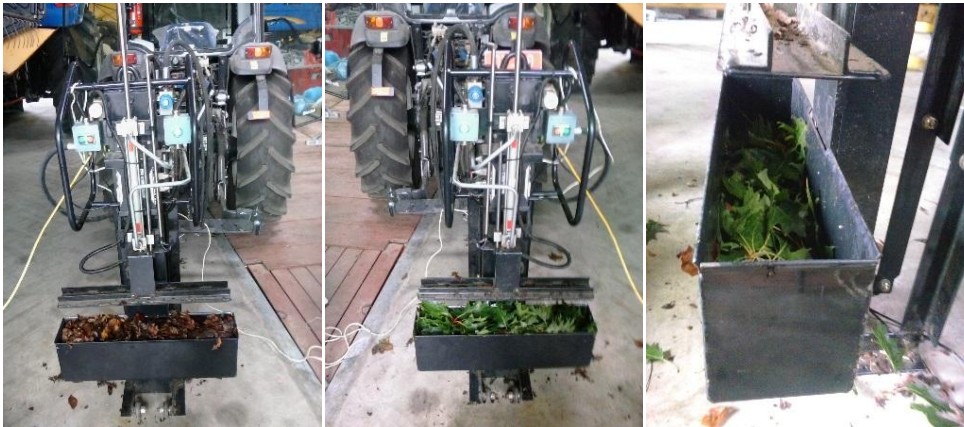
Figure 1 Compression box setup for material characterization of leaves (left), branches (centre and right)
