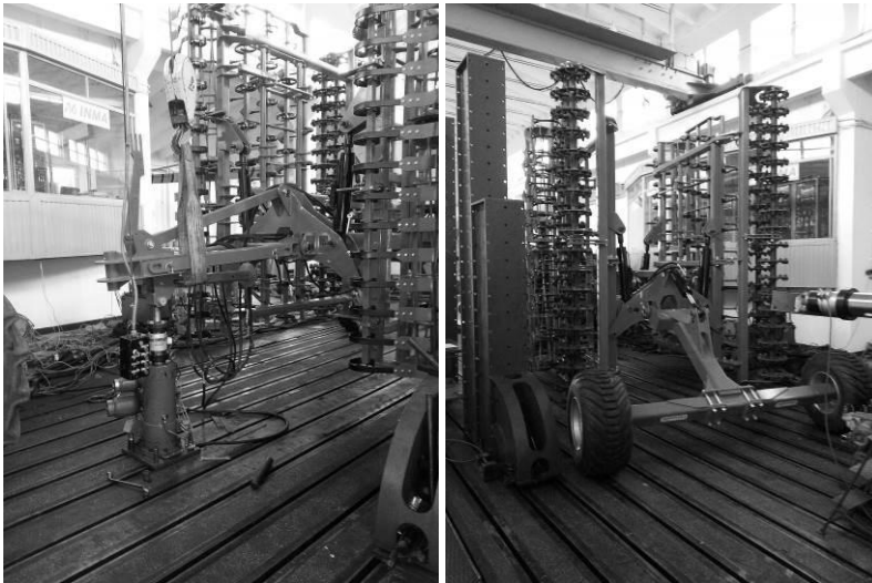
Fig. 4 Stand for testing in simulated and accelerated regime of agricultural combination implement in transportation conditions (left – in front view, right – view from behind)
