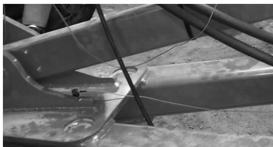
Fig. 1 Accelerometer mounted on the combinator's drawbar
