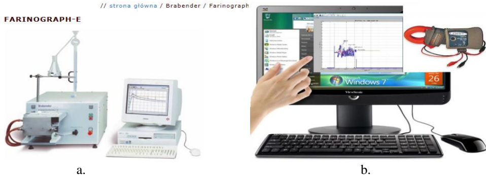
Fig. 1 a. Brabender farinograph; b. Portable device used for measuring the consumed current when kneading dough
