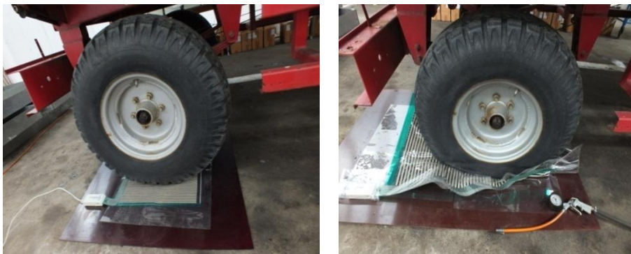
Fig. 4 Testing with maximum wheel load (21.18 kN), tire inflation pressure of 300 kPa (left) and 180 kPa (right)
