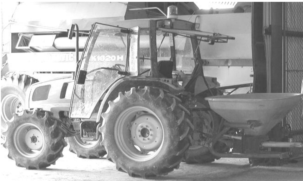
Figure 3: CREINA oscillating spout spreader coupled to tractor
