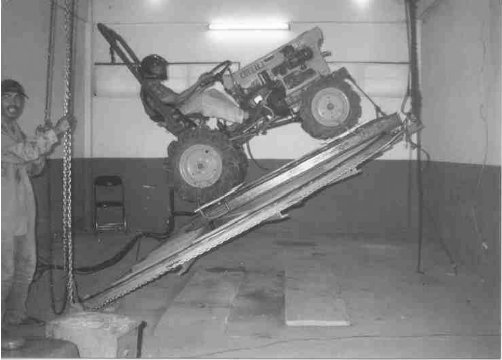
Figure 1: Testing in the laboratory on the tilting table for heading angle from 0 to 180 degrees
