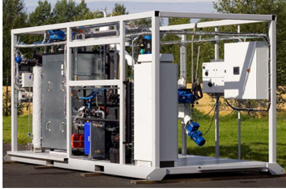
Figure 4. Volter 30 CHP facility before installation on the farm (Artim, 2014).
