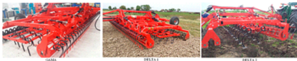
Figure 2. The prototype vibro-combinator SANDOKAN 2 equipped with the three types of active elements (GAMMA, DELTA1, DELTA2)
