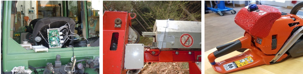
Figure 1. Here the three developed FDLs were shown: on the left the Tractor-FDL, on center the Yarder-FDL while on the right the Chainsaw-FDL. The Tractor-FDL is energy supplied by the electric circuit of the tractor, while, the others foreseen the use of external LiPo.
