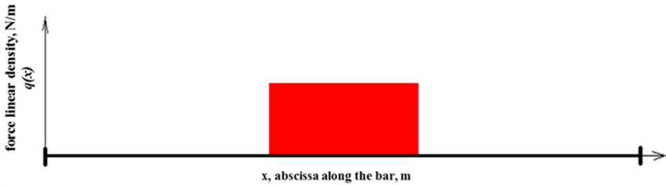
Figure 2. The geometric scheme of the linear force density distribution on the bar
