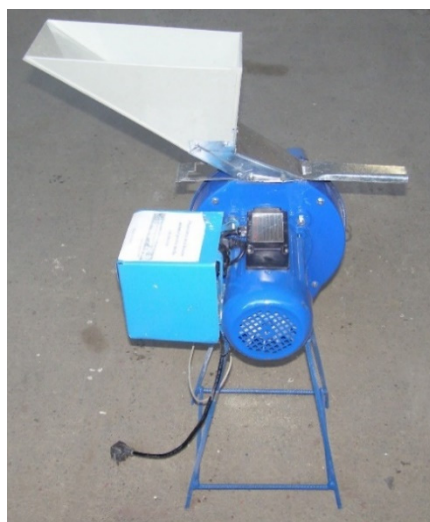
Figure 1. Modified universal household M.F KBE-250T mill
