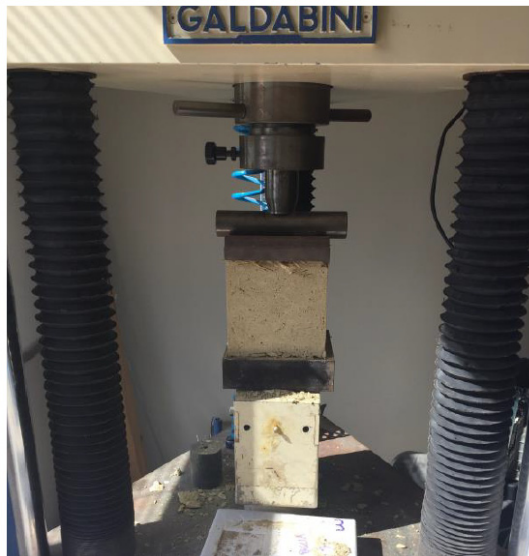
Figure 5. Compression test on an adobe bricks.
