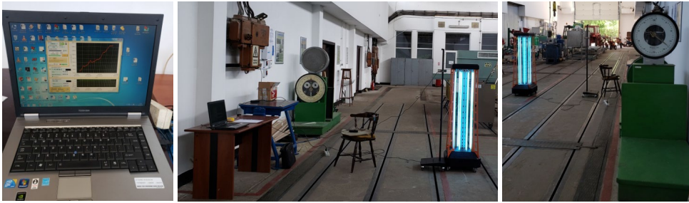
Figure 4 Determination of the intensity of UV-C radiation performed for the device for disinfecting surfaces within rooms
