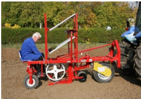
Figure 1 Working seedlings planter and kinematic scheme of the movement transmission from the drive wheel to the distribution disc with articulated buckets
