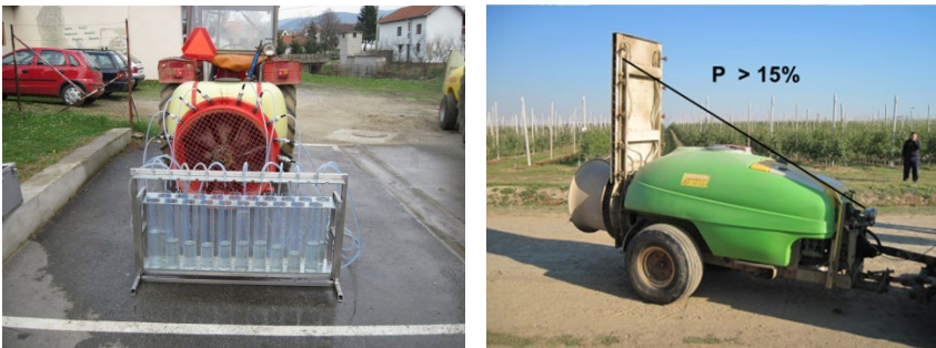
Figure 3 Nozzle flow check (left) and pressure differences check (right)
