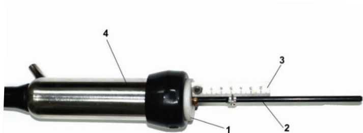
Figure 3 Measuring the mouthpiece depth 1-conical plug; 2-cylindrical rod; 3-ruler; 4-teatcup
