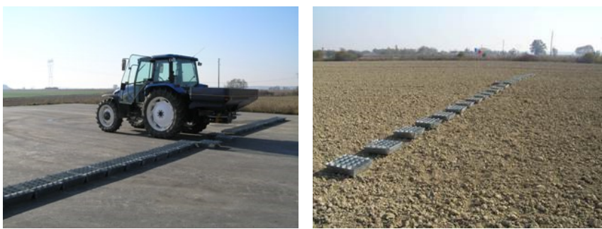
Figure 5 Mineral fertilizer spreader testing with test boxes
