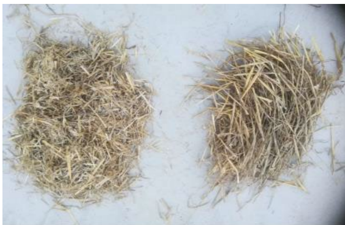
Figure 1 Straw after passing through a rotary (left) and conventional (right) thresher drum (photo: A. Zmaić)
