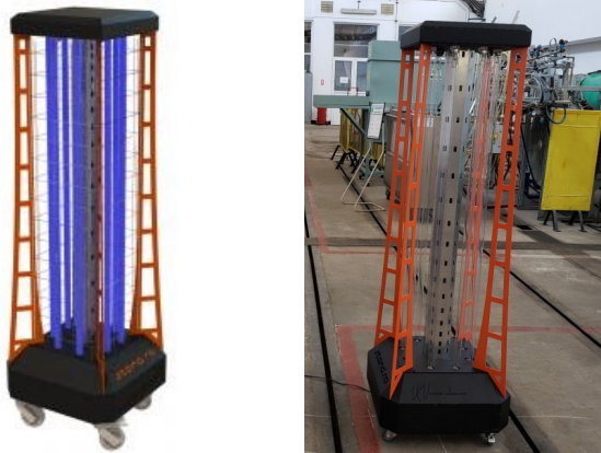
Figure 2 The portable UVC directed device for disinfecting the surfaces within rooms (3D model – left side; physical model – right side) ( www.stand.ro ; Sorica, 2020)
