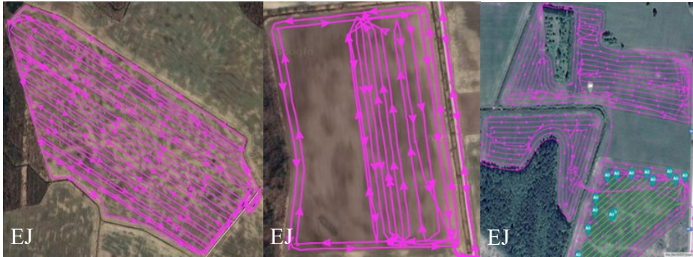
Figure 3 Field diagrams EJ4, EJ5, EJ6 when the combine is controlled by the operator, manually
