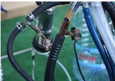
Figure 5 Absolute pressure sensors mounted on the short pulse tube and short milk tube
