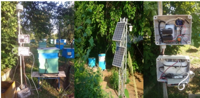
Figure 2 Meteorological station for measuring the microclimate in the bee colony and beyond
