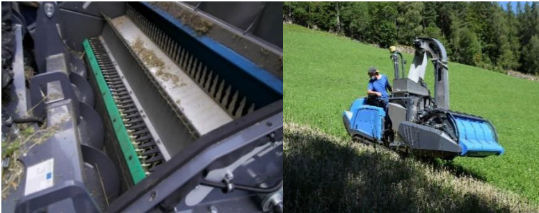
Figure 2 Stripping comb stripper head and conveying system (mechanic)
