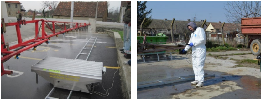
Figure 2 Surface distribution check with spray scanner (left) and individual nozzle flow check (right)
