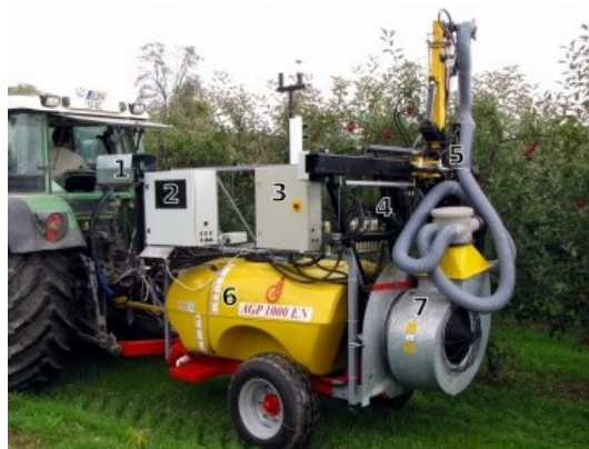
Figure 3 LIDAR sensors on orchard sprayer (Osterman et al., 2014)
