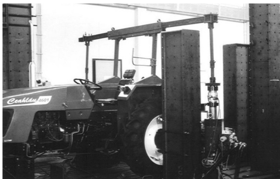
Figure 2 Mounting performed an "HIDROPULSE" installation for testing the welded frame, drive from the up to down
