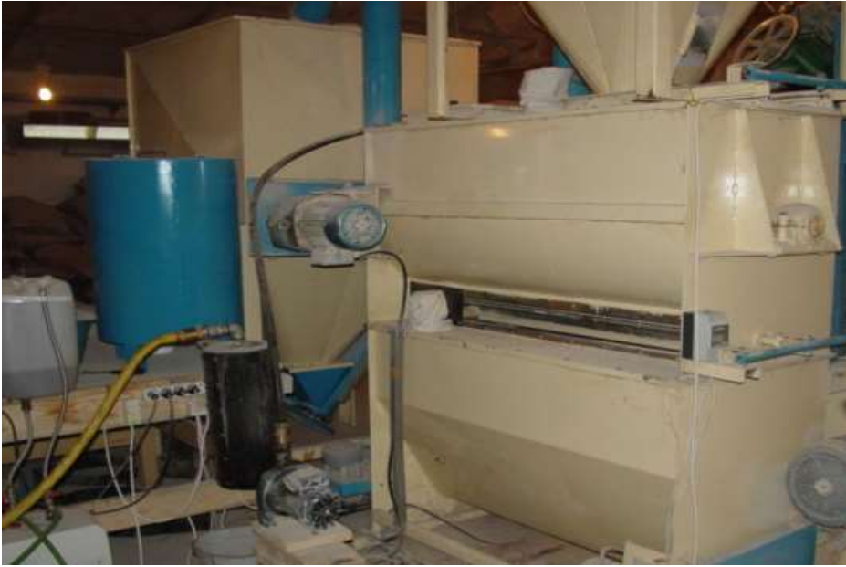
Photo 1 Horizontal dual ribbon mixer
