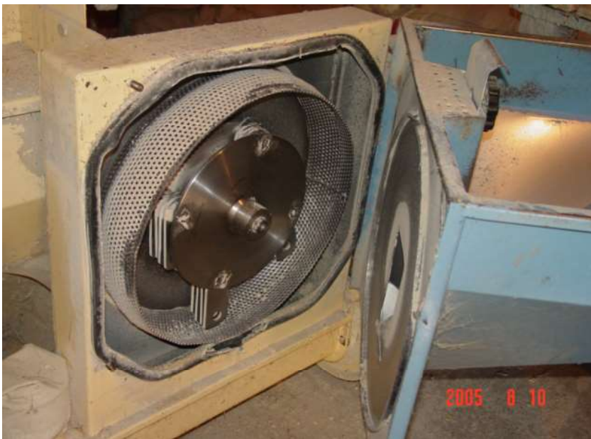
Photo 4 Hammer mill with 4mm screen
