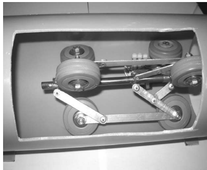
Figure 7 Picture of the developed in-pipe minirobot
