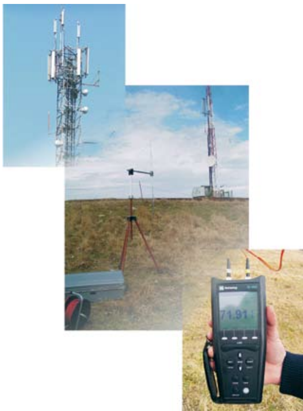
Electric field measurement of high power transmitters
