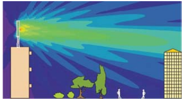
Electric field distribution of a typical GSM base station
