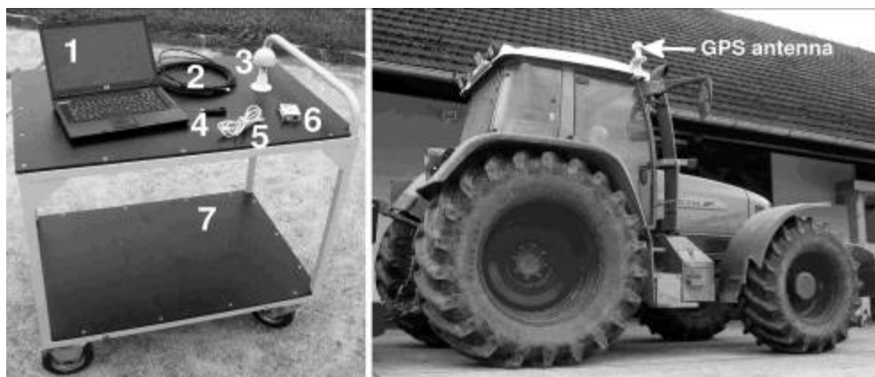
Figure 1 Laboratory rover (left) with laptop computer (1), antenna cable (2), GPS antenna with mount (3), USB GSM modem (4), USB cable (5), GPS receiver (6) and moving platform (7), rover for field testing is tractor-based (right)
